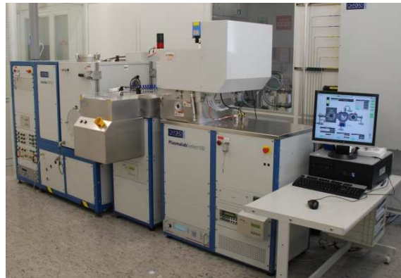
Reactive Ion Etching: Oxford Plasmalab System 100 with ICP 380 source
