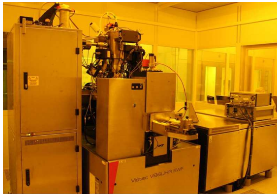
Electron-beam lithography: Vistec VB6 (100 kV)
